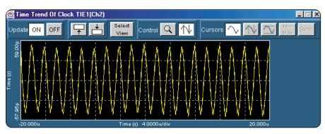
Figure 1. Time Trend of Clock with Sinusoidal Jitter.
