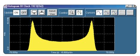
Figure 2. Histogram of Clock with Sinusoidal Jitter.
